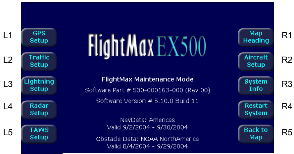
Figure 2: Maintenance Mode Main Page (actual view depends on installed options)
